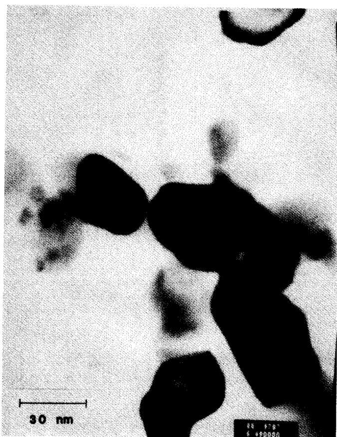
FIG. 2. TEM micrograph taken after 400°C hydrogen treatment of the FeRh/Grafoil sample.
