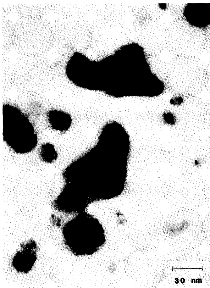
FIG. 9. TEM micrograph taken after 100°C reduction of the previously oxidized FeRh/Grafoil sample.
